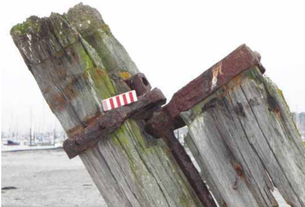
Figure HAM037- 4 The axel of the rudder comprises of a pin with a bracket fastened to the sternpost and the rudder stock (looking south)
