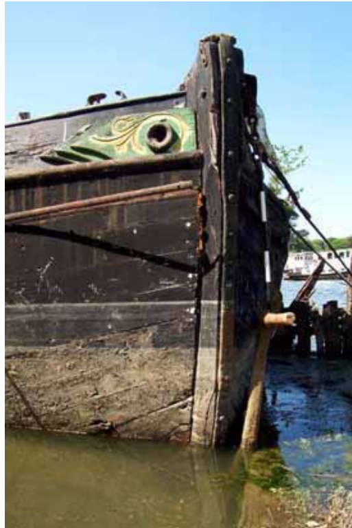
Figure HAM017- 4 Bow view with decoration around the hawse holes clearly visible
