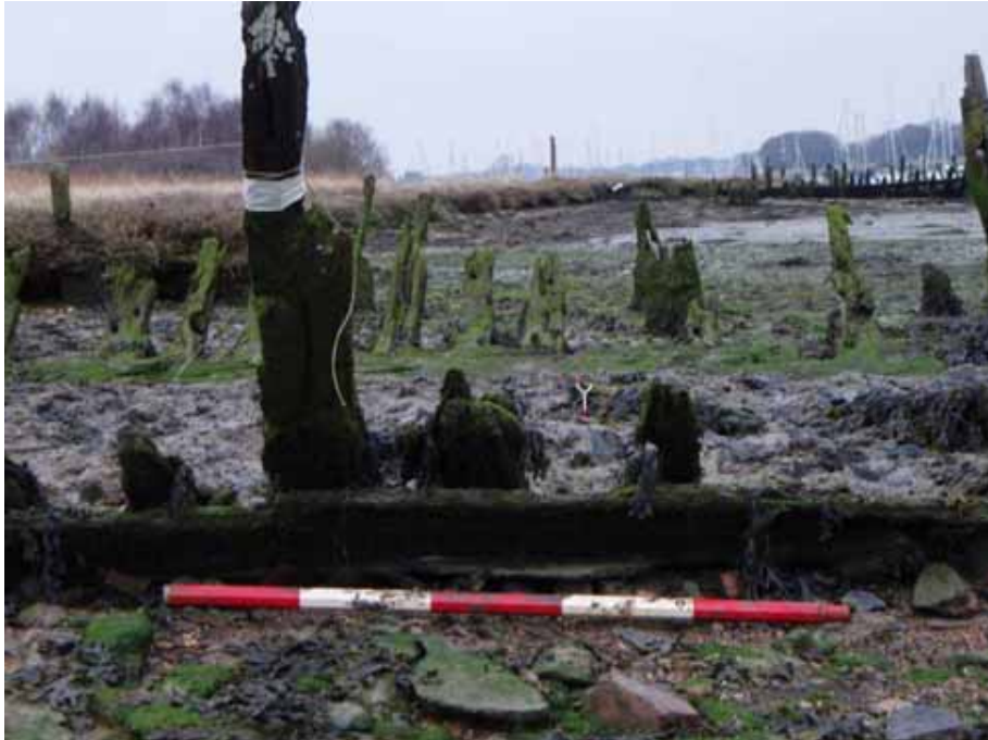
Figure HAM037- 7 A section of hull planking on the port side. It can be seen on this photograph that scouring beneath the vessel is occurring (looking north)
