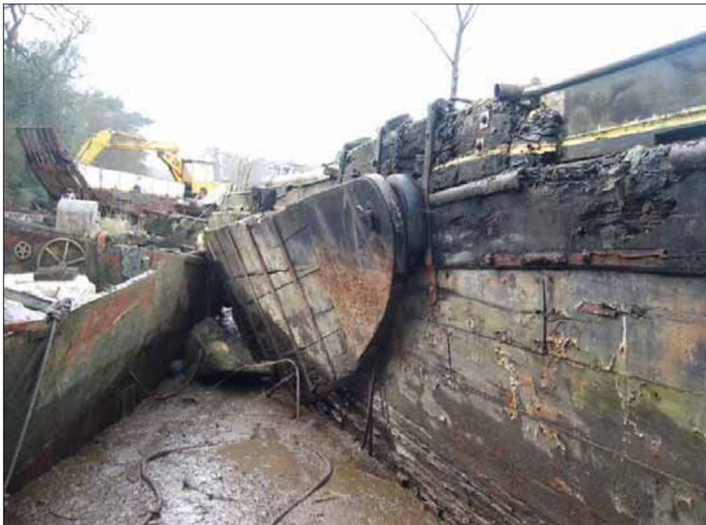
Figure HAM017- 6 Photograph of the starboard leeboard
