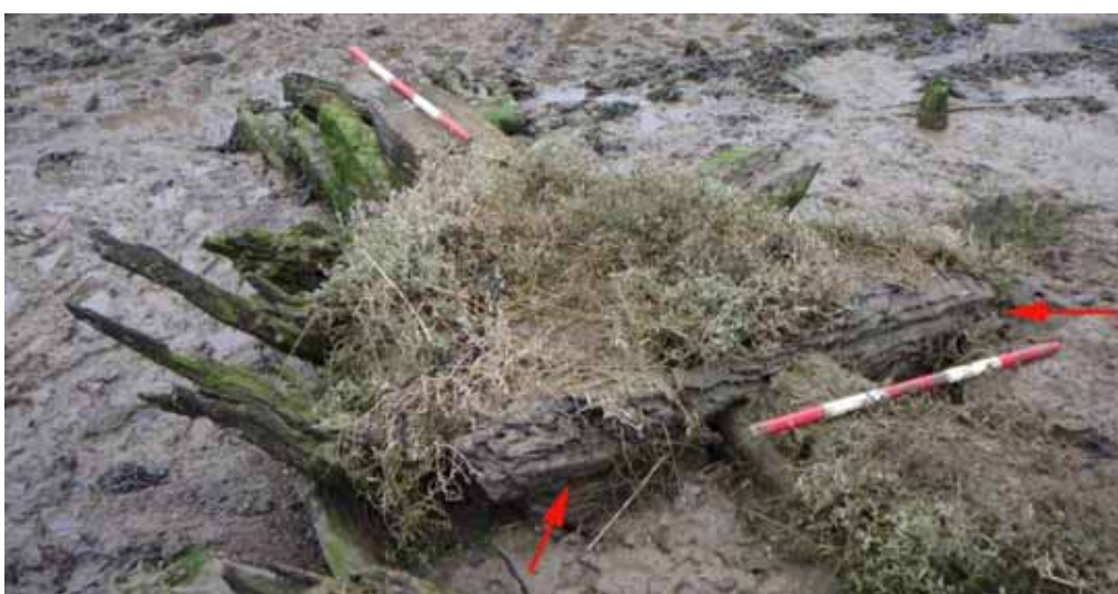
Figure HAM037- 10 The bow section of HAM037 with the concrete ballast indicated (looking northwest)
