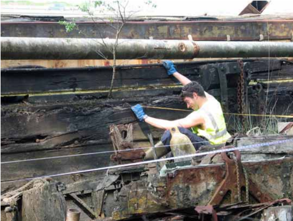
Figure HAM017- 1A student using the datum offset method of recording in somewhat uncomfortable conditions
