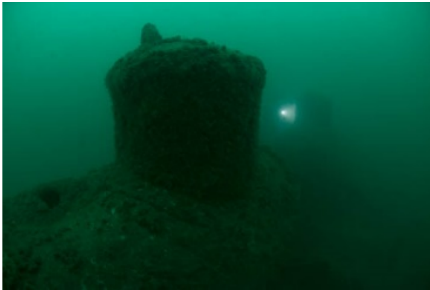
Figure 10: Steam dome on top of the boiler, a dome on top of a boiler behind can be seen in the distance (photo courtesy of Michael Pitts)
