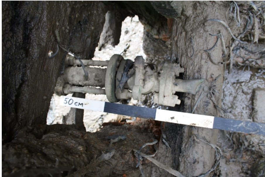
FIGURE 19 – INTERNAL SEA COCK / PUMP FITTING
