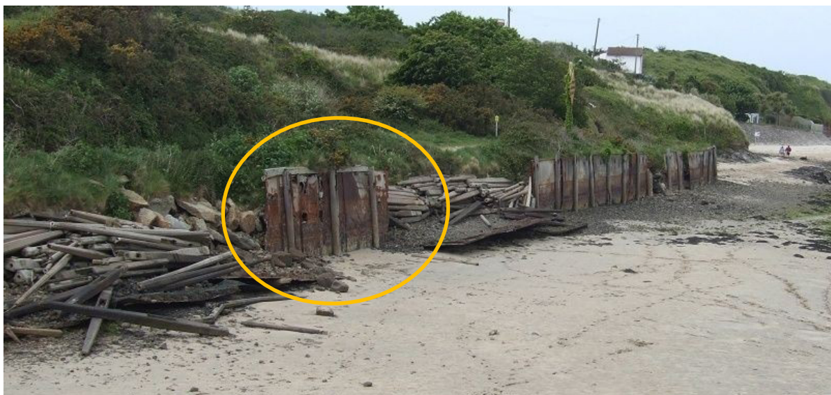
Figure 32: collapsed hull plating either side of a standing section, supported by 3 wooden stakes (Photo by Raymond Forward 2009)
