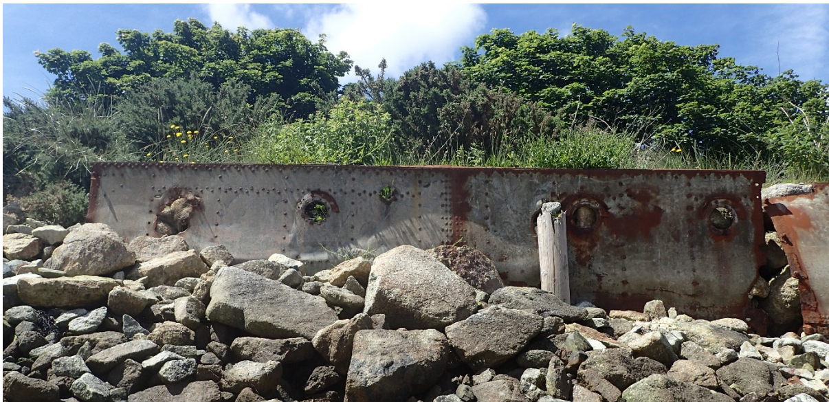
Figure 16: riveted panels of ship's hull (2016). Panel 8 to right, panel 9 to left.
