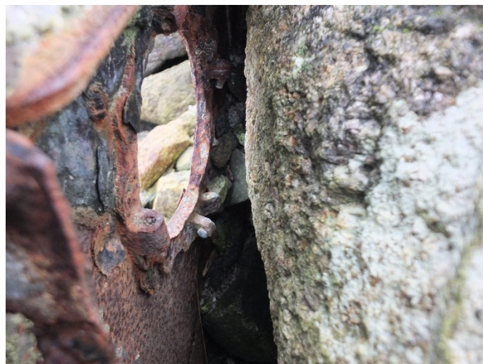
Figure 18: the rear/inside of a porthole - with remains of the hinge and locking mechanisms
