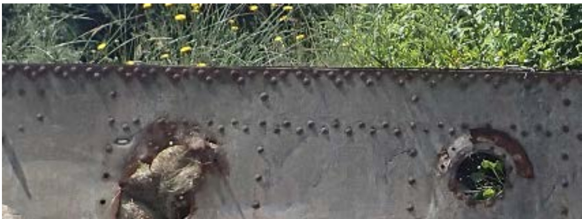
Figure 11: riveting pattern at the gunwale, panels 6 to 9 (2016)
